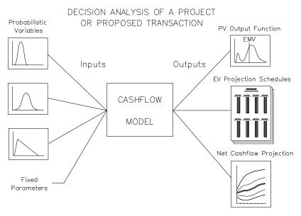
**Figure 1. Project Feasibility Forecast Model.** A deterministic net cash flow model is at the core. With even a single distribution input, the outcome will be a distribution.
