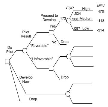
**Figure 3a. Schematic Decision Tree.** This is to evaluate whether to do a pilot flood on an oil field. *EUR* is the Estimated Ultimate Recovery. Amounts are in \$million.
